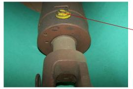
ALL ports on WYR-LOK cylinders are machined into the base casting AND the gland casting.
